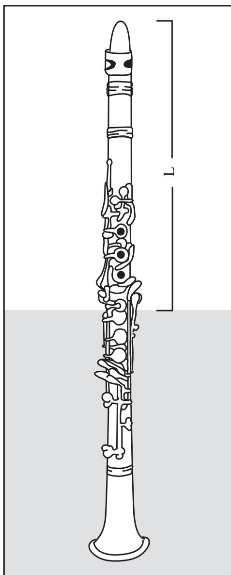
**Figure 12-2.** The “length” of the clarinet is from the mouthpiece down to the first noncovered hole. The region below the first noncovered hole (shaded in light gray) does not contribute to the pitch. *Note.* From *Musicians and the Prevention of Hearing Loss* (1st ed.), by M. Chasin, 1996, Clifton Park, NY: Delmar Learning. Reprinted with permission of Delmar Learning, a division of Thomson Learning.
