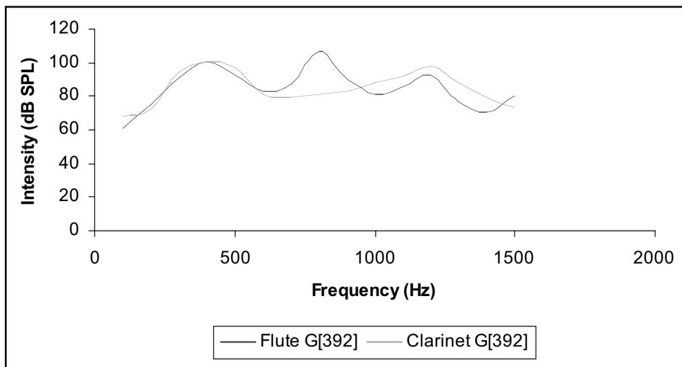
**Figure 12–3.** This shows the clarinet (a quarter wavelength instrument) and a flute (a half wavelength instrument) playing the same *concert* note (G[392]), normalized for playing intensity, demonstrating the differing resonant structures. The flute has twice as many resonances in any given frequency range as does the quarter wavelength resonator, the clarinet.
